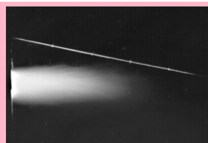
Gas (left) and light oil flames for 6514-6 Dual-Fuel Burner with 16 osi main and atomizing air pressure drop across burner. White lines on pipe above flame indicate 1' intervals.
